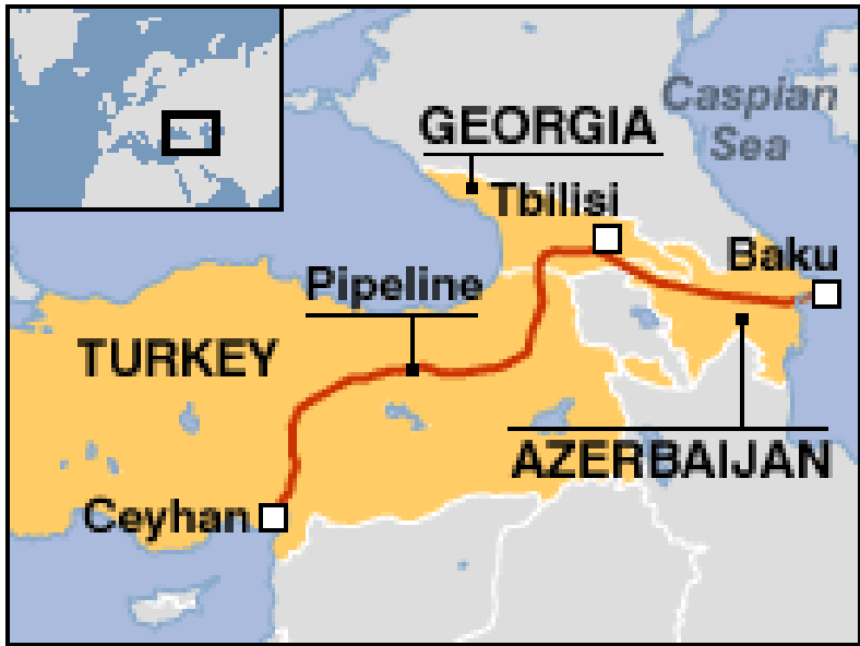
Baku-Tbilisi-Ceyhan (BTC) Pipeline. Source: BBC.co.uk
